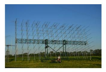
This is his 432 MHz EME antenna. It is made of 128 11 element yagi beams (all home made, designed by a friend of his). This means its a 1408 element antenna. It offers about 33.7 dB gain over a dipole. THAT MEANS: If you feed it with 1000 watts, you get an ERP of 2,370,000 watts.
