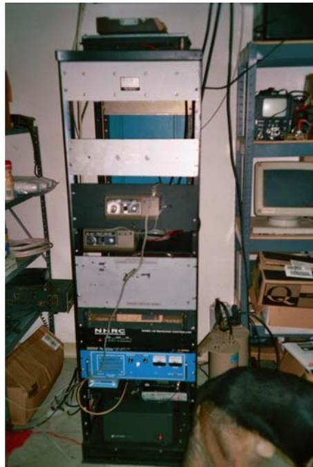
**KS1R 147.21 and 444.4 MHz repeaters + APRS & packet nodes**
