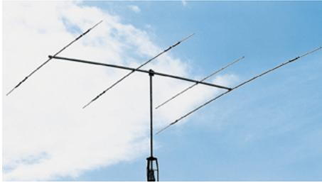
**2-Meter 13-element Long John Yagi**, including the complete mast assembly
