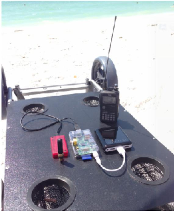
Check out Bryan's setup. What you see in the picture is a rechargeable supply for charging USB devices. Its powering a Raspberry PI in a case running software to connect to our D-Star repeater from the DVAP. I'm not sure where the internet access was coming from but perhaps the hotel's Wifi. Nice setup Bryan!
