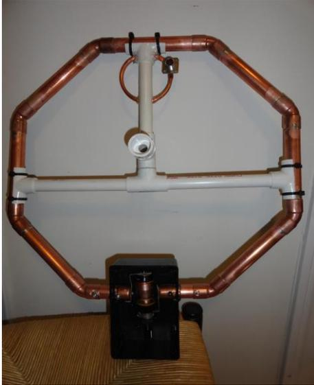
I housed the tuning cap in a 3.5 x 6" Radio Shack plastic project box and sealed it up with silicone caulk to keep it weather tight
