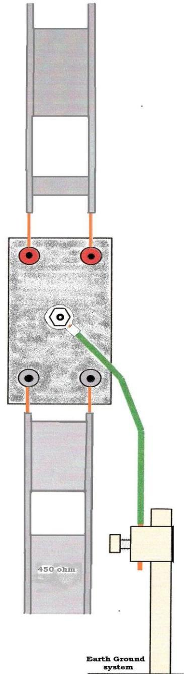
The arrester should be placed within a few feet of the ground rod (+ bonded ground system). The ground lead (made from #10 or larger copper wire or solid copper strapping) and should be as close to a straight line as possible.
