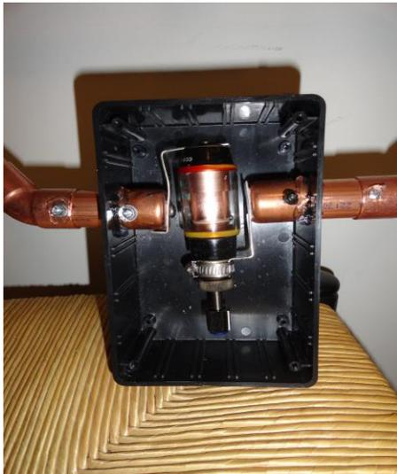
This plumber's dream antenna will replace my old aluminum folding chair squalo loop on the side of my tower sometime this summer/fall. It will be mounted horizontally for omnidirectional performance, as was the old squalo. It could be mounted vertically but the radiation pattern would be in the shape of a figure eight, like a dipole.
