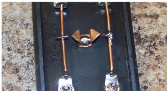
In the above snapshot you can see a small cat's whisker wires soldered on the through conductor on each side next to the cathode. They facilitate an easy point to point arc path. I used solid #20 for the cat's whiskers.
