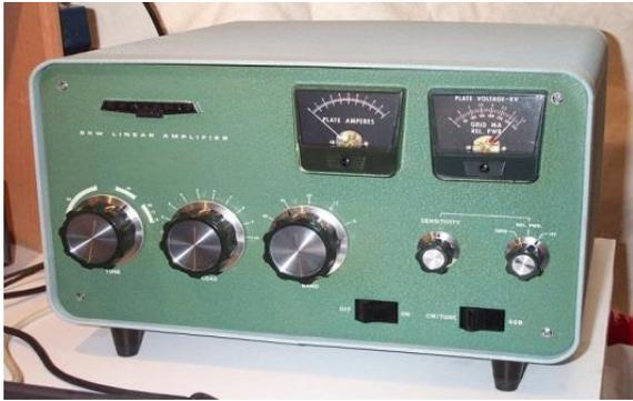
**Heathkit SB-220 HF linear Power Amplifier** (original, unmodified) with a pair of 3-500Z final tubs giving you a true KW (2 KW PEP). He was going to modify it for a 6M KW amp but never got around to it. **Asking \$400** with pick up at W1ZE's QTH in Phippsburg.
