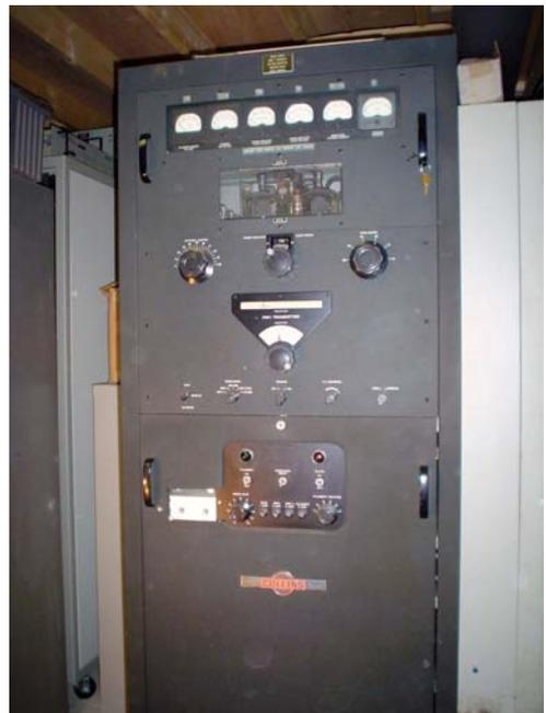
The above picture is of a Collins KW-1 transmitter. It is owned by N4LEM in Cocoa, FL. where I do voluntary work on ham gear and broadcast equipment. Go to: [www.isquare.com](http://www.isquare.com), Click in the lower left column, "Are you an amateur radio operator?" Up will come WOYVA's collection of 6 of these rigs. There were only 150 of them made, WA1IE, Chuck in Waterville has one. Runs 1 KW input. **73's, Pete K1MJP**
