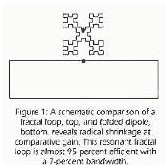
Those that are hyping fractal antennas—most notably W1YW, CEO of Fractal Antenna Systems—claim several advantages. These advantages purportedly include wider bandwidth and smaller size when compared to traditional antennas, such as verticals and dipoles. Those that are trying to debunk these claims contend that this is all just hogwash, and that there's no real scientific basis for these claims.
