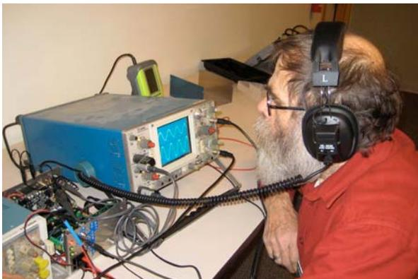
The device, especially useful for CW operation, consists of two filter amplifier-processors that when listened to with a good set of
