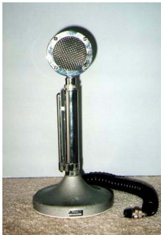
However the newer solid-state SSB transceivers have lower microphone impedance, in the neighborhood of 600 ohms. When you try and use a D-104 with these rigs, the audio tends to be constricted and a bit tinny. Because of this, some hams have replaced the internal ceramic microphone element with a 600-ohm dynamic element. That works well but to the purest, the microphone is no longer a true D-104.
