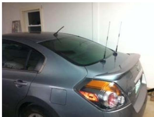
Recently I purchased an IC-2820 for my car. I couldn't help but notice there were two antenna ports on this radio and further reading showed I could optionally connect a second antenna for diversity receive. In short diversity receive is the ability of the radio to choose between two antennas the one with the strongest receive signal. But is it worth the effort?
