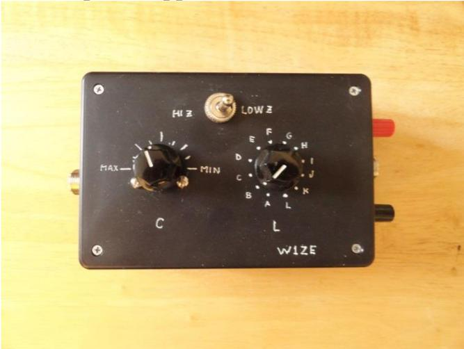
The tuner has a minimum of parts and I assembled it in an afternoon in my very small workshop here in Poway, CA. This tuner is capable of handling 100 watts and works well with random and long wire antennas but can be used with coax fed antennas also. Since it is small it makes a nice portable tuner for field activities.
