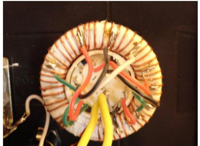
In the above photo you can see the T200-2 toroid first wrapped with a layer of teflon plumbers joint tape. This will keep the toroid from rubbing off the enamel on the coil wire and provides some insulation if any arcing occurs. Next I space wound 45 turns on No.20 enamel magnet wire on the toroid.
