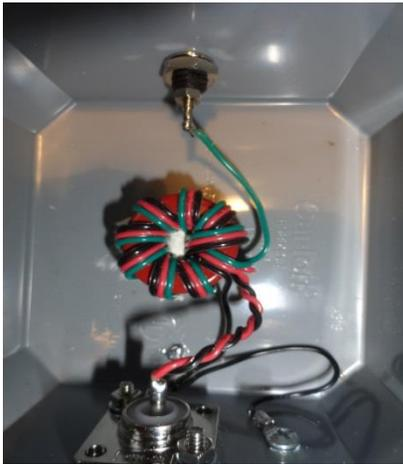
All that is needed is to connect your end fed wire and check it out. It is recommended that wire lengths of 24.5, 36 or 55-feet in length seem to work best for 40 to 6 meters with an SWR 3:1 or less.
