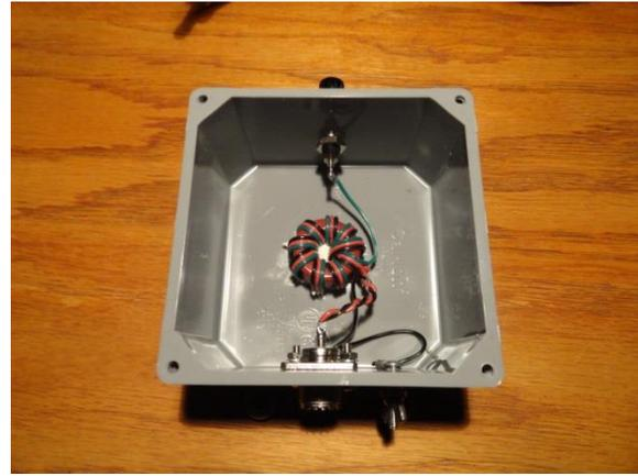
I collected all the parts needed and built a 9:1 UnUn and housed it in weatherproof plastic electrical outlet box and just added a few extra parts like a SO-239 coax connector, an antenna binding post and some stainless steel hardware. Winding the toroid transformer was east and only took a few minutes
