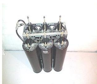
which is a must have for our repeaters. Plus the two additional cavities will increase the 600 kHz split isolation and narrow up the
