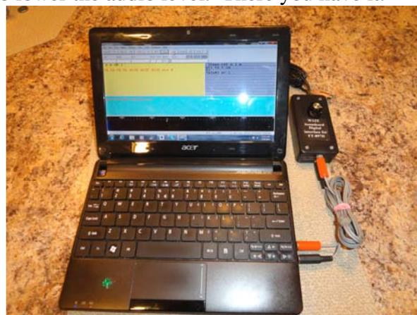
The isolation transformer arrangement in last months newsletter can be used and this little keying circuit can go into the same plastic interface box used to house the existing transformer that couples the transmit/data audio from the laptop to the transceiver.
