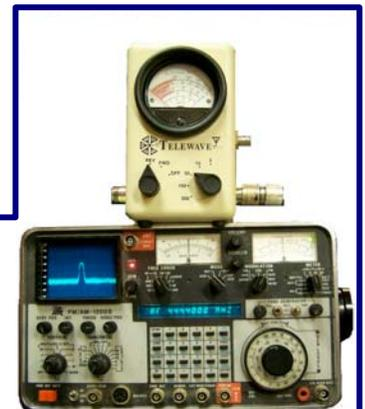
K1MNW's IFR-1200 service monitor and Telwave 30-1000 MHz wattmeter used to do diagnostics
