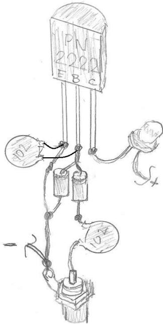
I used a BNC connector for the antenna/probe input but a cheaper RCA connector should work fine. The entire circuit including battery holder can fit into a small plastic project box.
