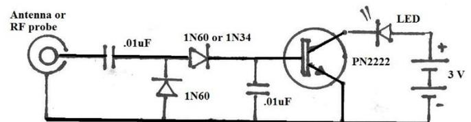
The two rectifying diodes can be either 1N34s or 1N60s. 1N914 or 1N4147 can also be used if that is all you have. The NPN transistor can be any of the general-purpose type, such as the PN2222, 2N2222, 2N3904, etc. For my sniffer I obtained a
