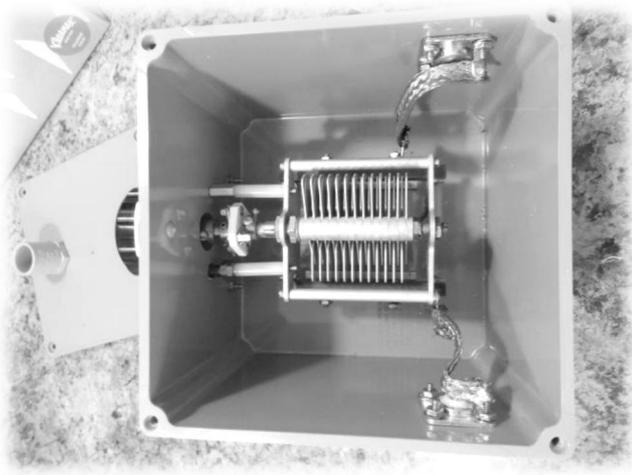
The antenna loop is connected to the capacitor tuning box via two SO-239 chassis mount connectors. Antenna radiation comes from the shield of the coax loop but I shorted the center conductor to the shield side of the SO-239s. I then connected on SO-239 to the stator terminal on the capacitor and the other SO-239 to the capacitors rotor connector using copper braid from a six inch length of coax.
