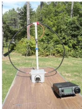
I had such a good time building the loop I wanted to try a minor mod to the design. That being replacing the RG213 antenna loop(s) with 3/8 inch soft copper tubing. The 3/8-inch size will fit nicely into the rear of the standard PL259 connector and could be sweat soldered in. I decided on a length of six foot and with the value of the tuning capacitor in the tuning box it would cover 30 through 10 meters.
