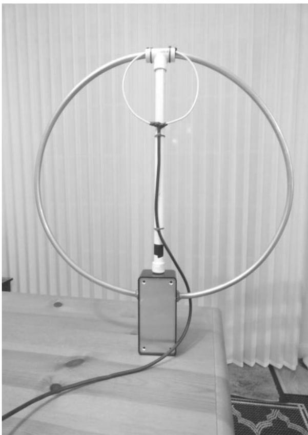
I drilled a 3/8" hole on each side of the plastic box about 2/3 the way up on each side so the copper loop ends could just pass through and be hot-glued in place. Then I hot-glued the the capacitor to the inside bottom of the plastic box. I used copper braid taken from a short length of RG-58 coax to make the jumper connection from the copper pipe loop ends to the capacitor (see photo).
