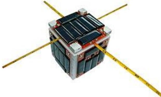
The spacecraft's name recalls the Amateur Radio call sign of Jordan's late King Hussein, JY1. JO-97 carries a 435/145 MHz SSB/CW inverting Amateur Radio transponder and a Slow-Scan Digital Video (SSDV) system to transmit stored images.
