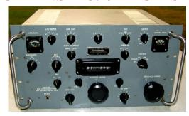
The Collins R-390A is a general coverage mil-spec MF & HF communications receiver capable of receiving AM, CW, FSK, SSB(with BFO) signals. Its tuning range is
