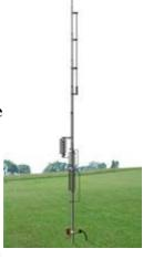
bands as the old HF6V. The 26.0 ft. tall Butternut vertical, is resonant on 80, 40, 30, 20, 15 and 10 meters and will easily handel 1,500 Watts PEP/CW, 375W Digital.
